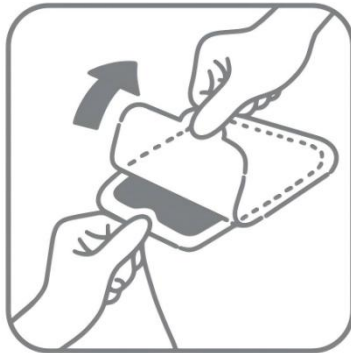
Figure 4-6 Separating pads from plastic liner
